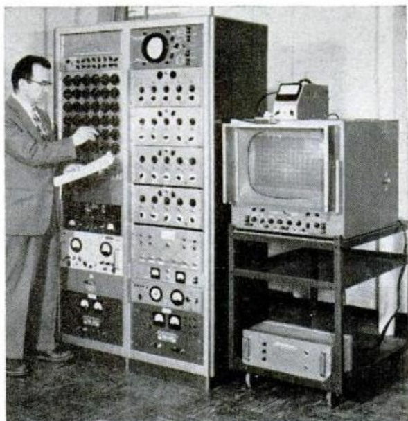
KNOBS ON PANEL insert bomb and weather data, and TV-like cabinet shows fallout pattern at once. Predicting it formerly took 15 minutes with high-speed computers, half-hour by hand.
